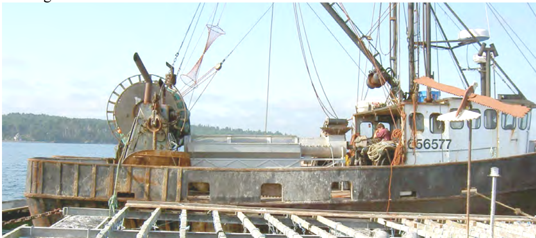
Figure 12. An Atkinson and Bower seed grader to grade seed into small, medium and large sizes, outfitted to a fish dragger. If seed is graded, keep the different sized seeded lines in different designated areas of the raft because they will be ready at different times of the year.
