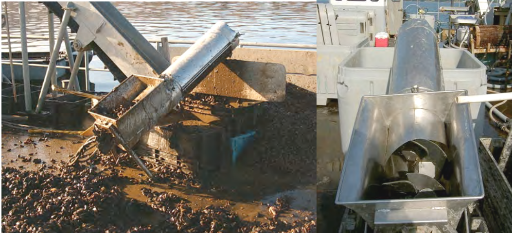
Figure 11. Mussel seed graded through an Aguin declumper either on deck or into x-actic totes. Note the correct angle of the declumper. Seed can also be washed by running a deck hose into the front of the machine.
