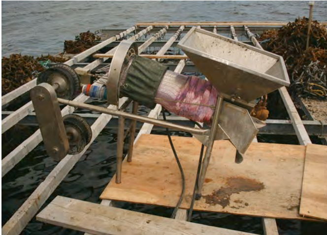
Aguin Seeding Machine using biodegradable cotton
